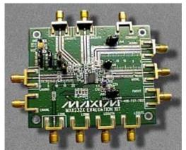
*Objective: To develop a suitable pair of 110MHz IF matching circuits for this chip on-board application of the cellular-band dual-mode CDMA front-end IC.*
